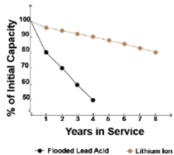
Battery Capacity Years in Service
